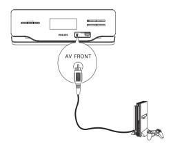
You can connect the AV output jacks on a game console to the AV1 IN or AV2 IN jacks on the main unit.
